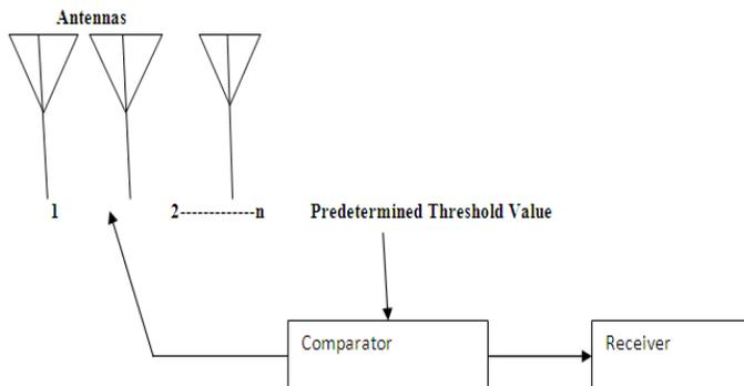
Figure 2. Block Diagram Of Feedback/Scanning Diversity
