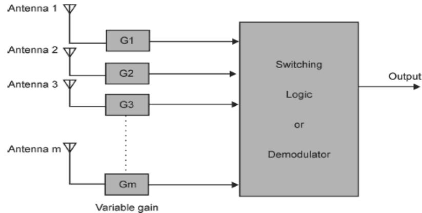
Figure 1. Shown the block diagram of selection diversity in communication systems.
