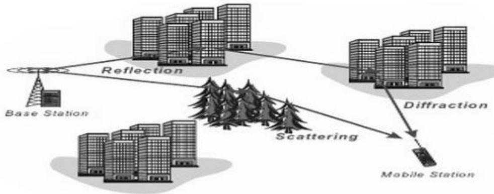
Figure 1: Multipath Signal Environment and Selection of strongest signal
